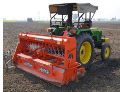
Figure 9: Roto till drill
