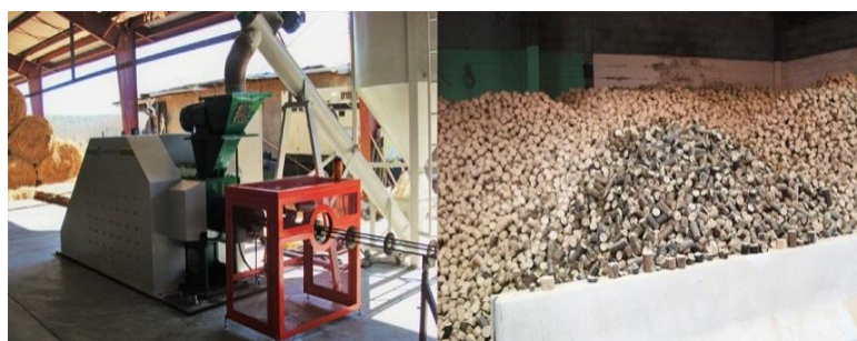
Fig. 25 (a) Pellet making machine (b) Prepared pellets
